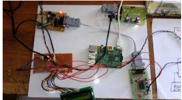
Fig3: display and initialized gsm and status If any rfid activated then microcontroller automatically excute the program. Calculate gps values and location and sends messages to predefine numbers in system. this process show in fig3 and alert message in fig4
